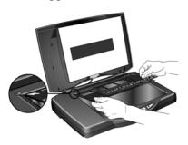
The 35mm negative holder also has a calibration slot next to it. Do not place items to be scanned in the calibration slot.
